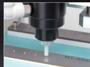
Tightens screws as small as M1.0.
